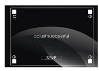
Press ADJUST SCREEN to display the above menu, there are a square button in the top left corner. Press the square button at place ①, then the button will move to place ②, press it at place ②, it will move to place ③, then place ④, press SAVE at last.
